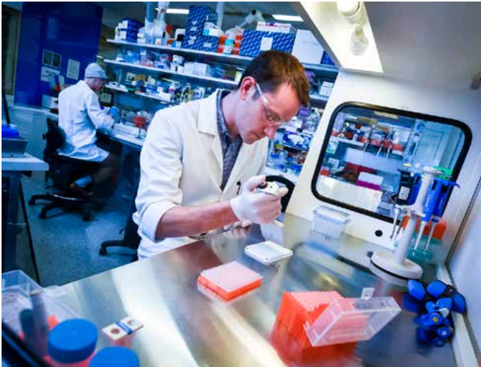
Testing for platypus DNA. DNA from a river water sample is extracted in the laboratory so it can be analysed to look for any platypus DNA that may have been washed downstream.
